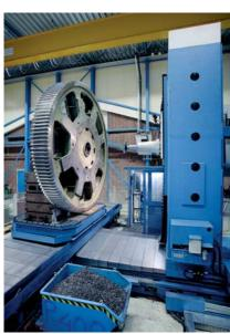
bevelling and flank line barrelling, are also made during the cutting process. Stork Gears & Services is able to produce high-accuracy gears for high-speed gearboxes as well as high load gears for durable applications (often in combination with multiple gear corrections).
